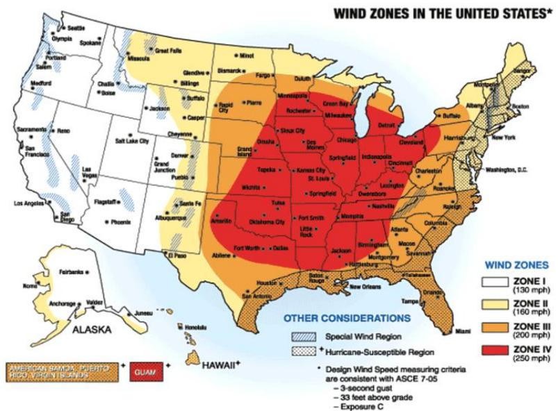
Figure 1A – Safe room wind speed map 2015 (courtesy of the ICC).
